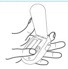
Start with the meter off (no test strip inserted). Open the battery compartment on the back and press the SET button.
